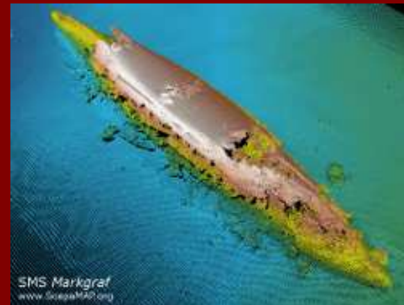
Sonar mapping – wrecks of German High Seas Fleet, scuttled Scapa Flow, Orkney, 1919.
